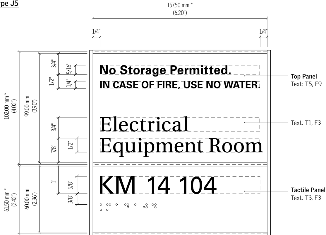
2 Detail Elevation - Sign Type J5 6" = 1'-0"
