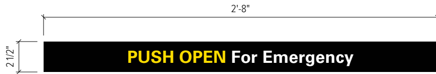
2 Elevation - Sign Type W10 (Door Side 2) 1 1/2" = 1'-0"
