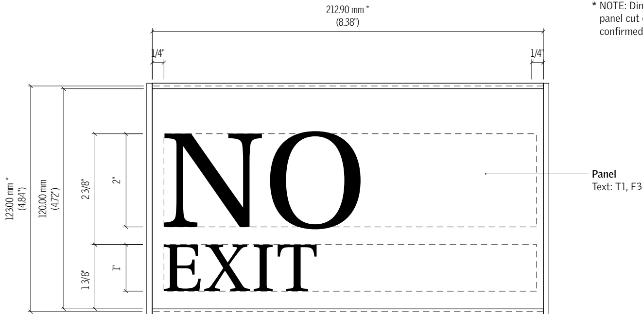
2 Detail Elevation - Sign Type U4 6" = 1'-0"
