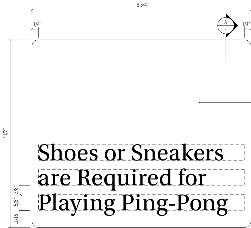
1 Detail Elevation - Sign Type W1.s 6" = 1'-0"
