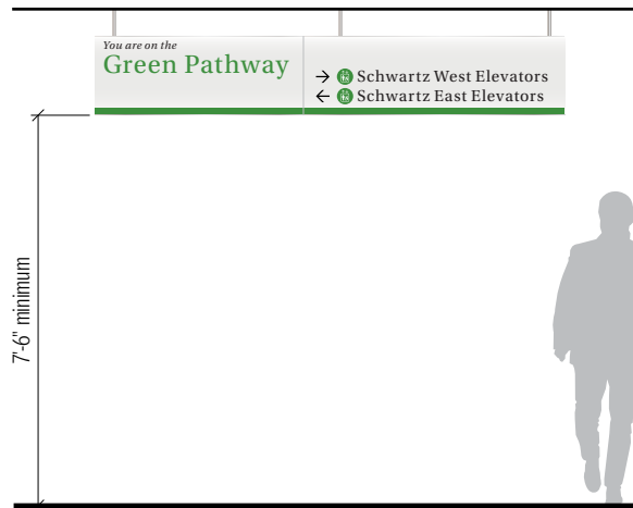
3 Installation Elevation - Suspended 1/4" = 1'-0"
