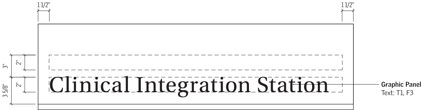
1 Detail Elevation - Sign Type E3a 1 1/2" = 1'-0"
