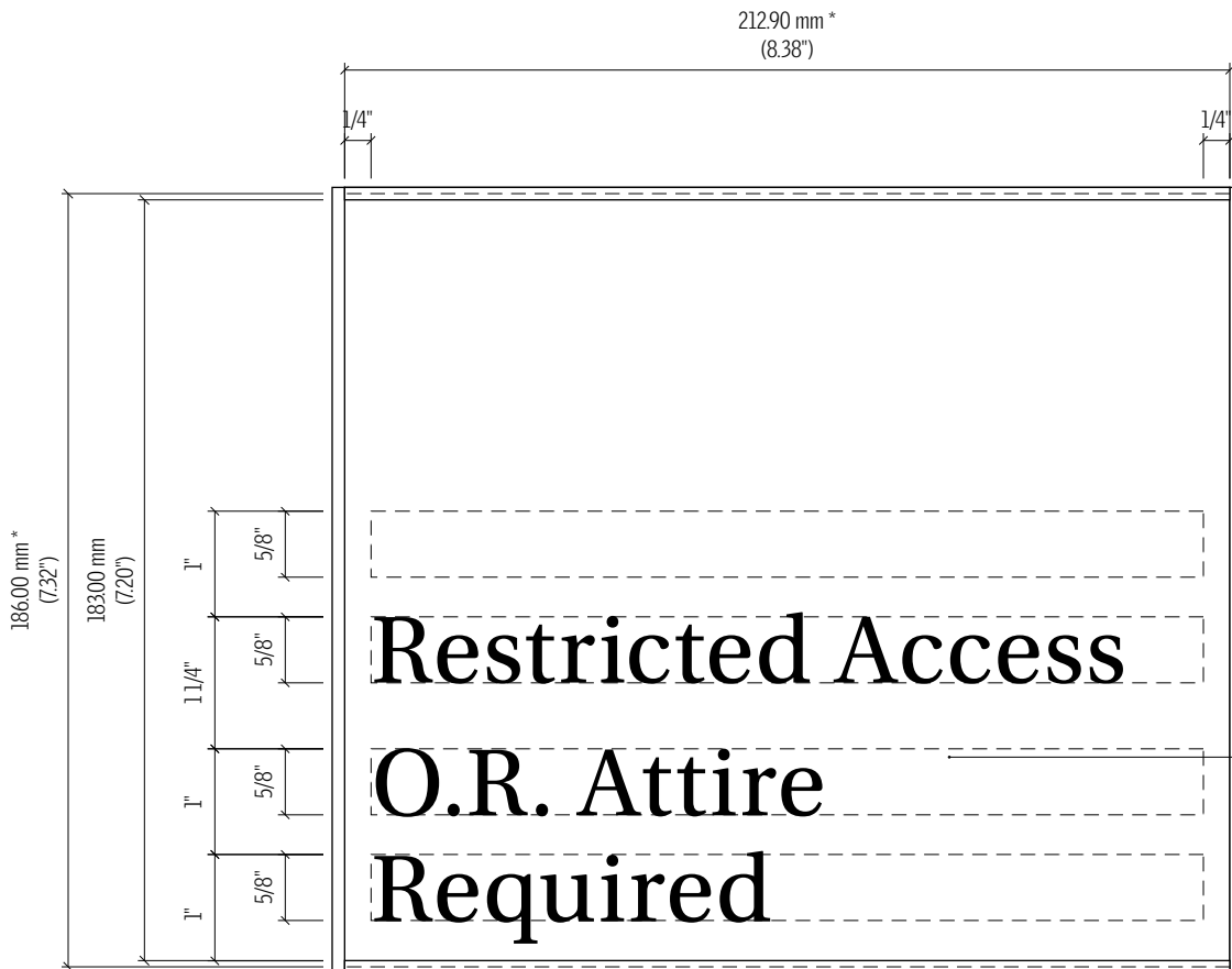
1 Detail Elevation - Sign Type W1 6" = 1'-0"
