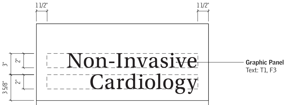
2 Detail Elevation - Sign Type E9a (Side B) 1 1/2" = 1'-0"
