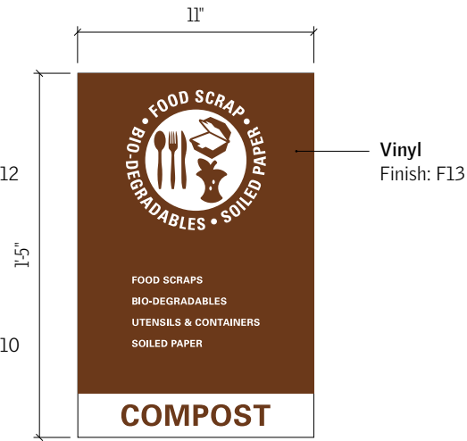
3 Elevation - Sign Type W20 1 1/2" = 1'-0"
