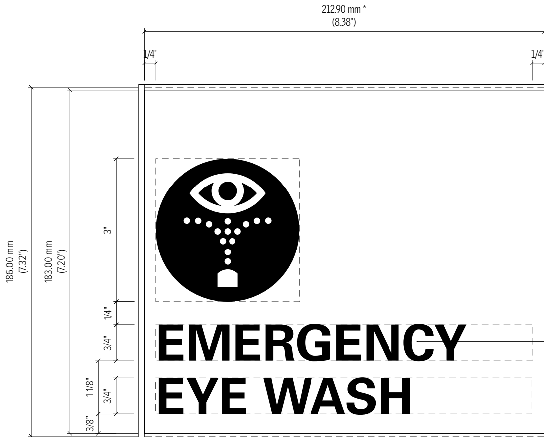
1 Detail Elevation - Sign Type W1 (Eye Wash) 6" = 1'-0"
