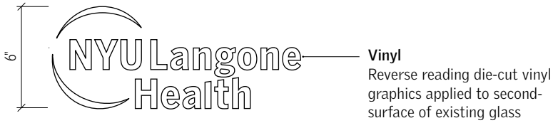
2 Detail Elevation - Sign Type VV1 1 1/2" = 1'-0" Finish: F66
