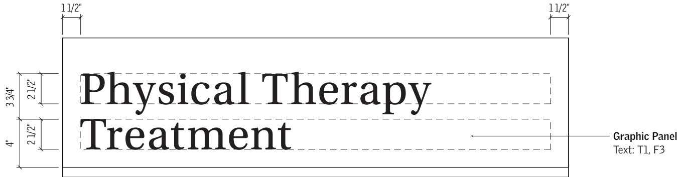
1 Detail Elevation - Sign Type E3b 1 1/2" = 1'-0"
