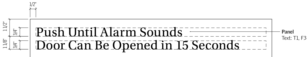
3 Detail Elevation - Sign Type W3 3" = 1'-0"
