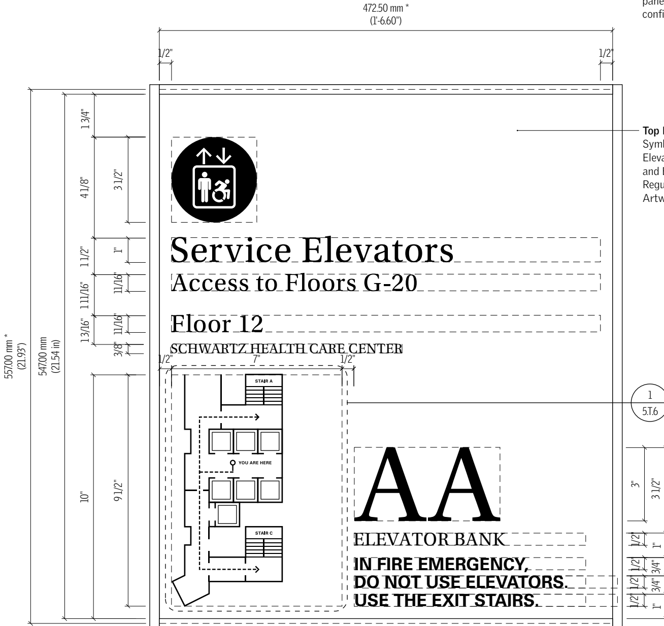
1 Detail Elevation - Sign Type T2a (Alternate Layout) 3" = 1'-0"
