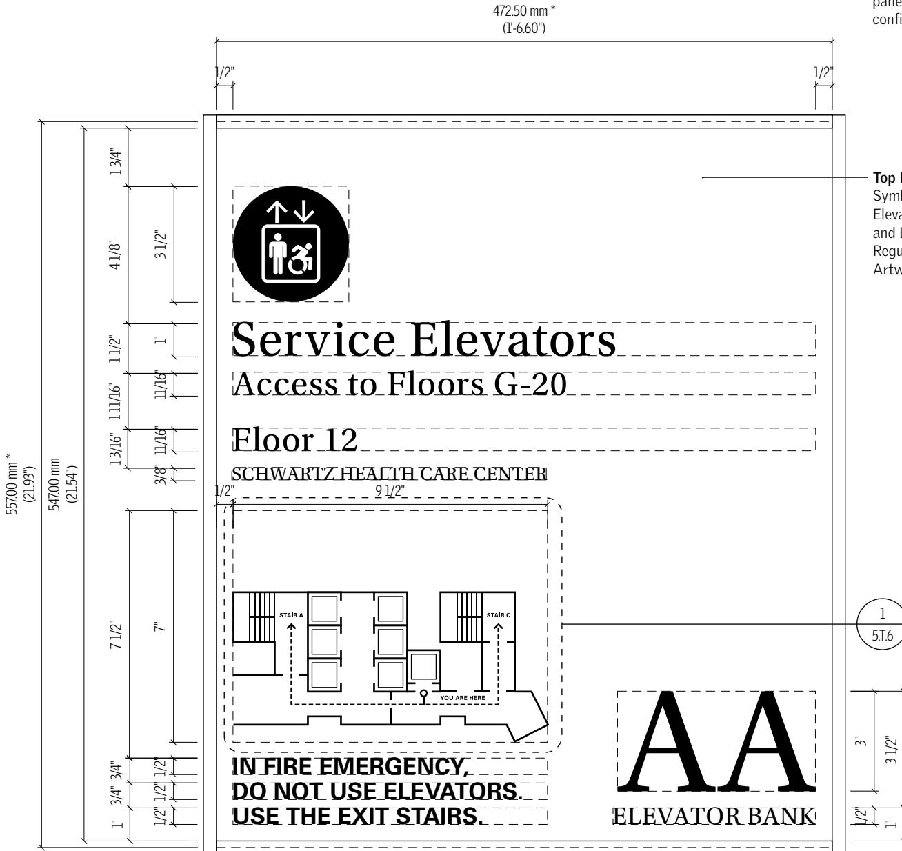
1 Detail Elevation - Sign Type T2a 3" = 1'-0"
