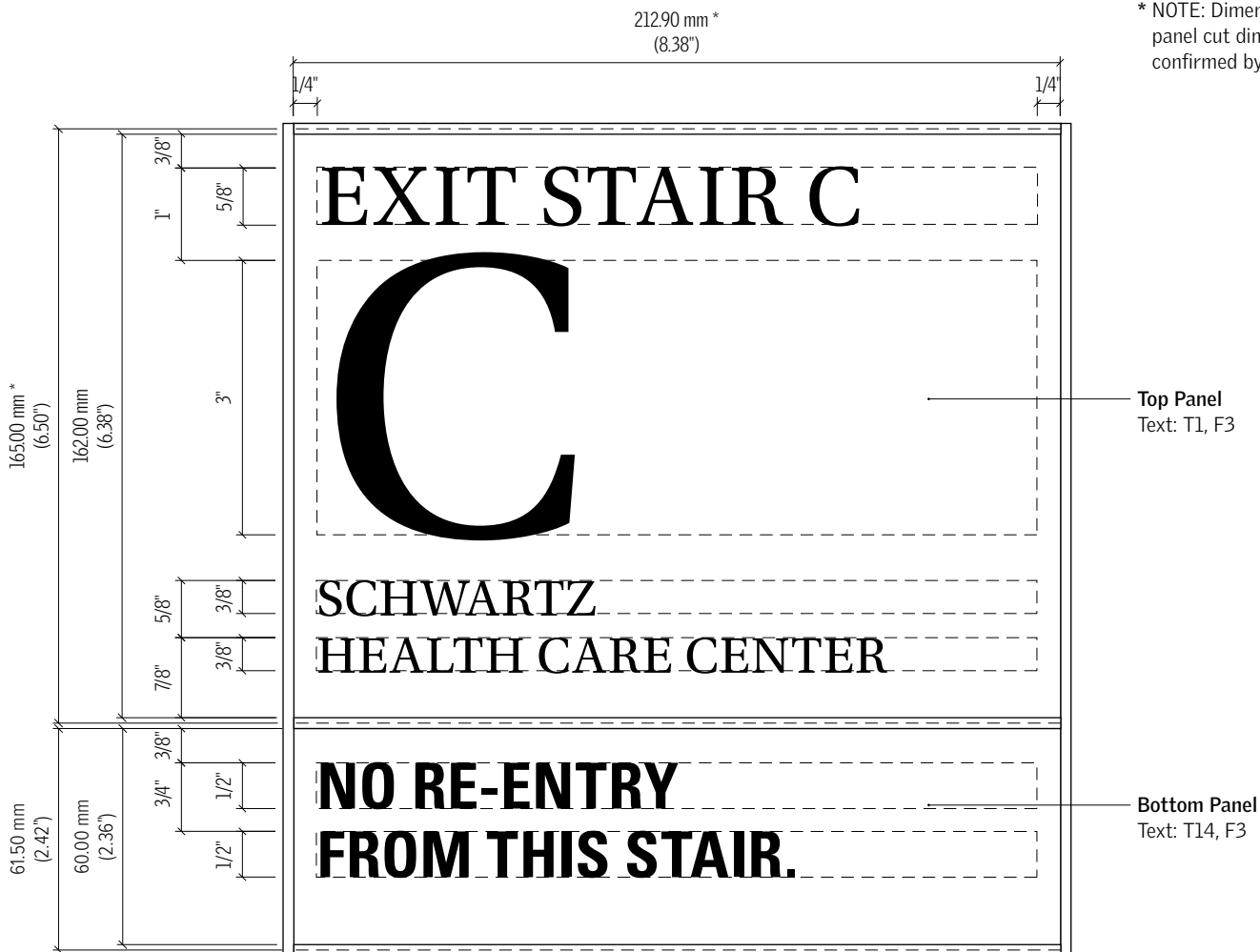
1 Elevation - Sign Type U1b 3" = 1'-0"
