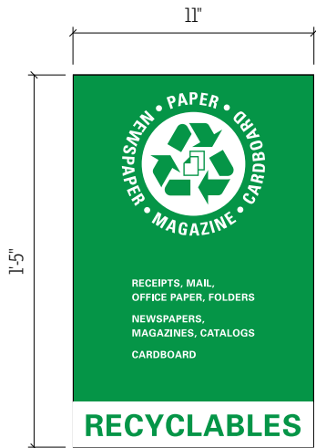
1 Elevation - Sign Type W20 11/2" = 1'-0"
