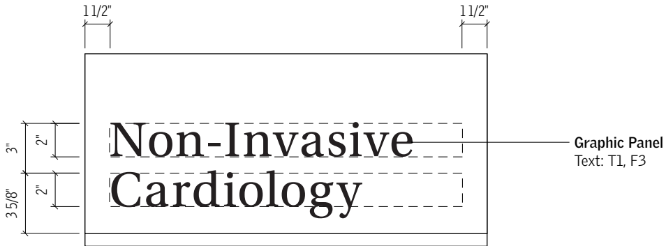
1 Detail Elevation - Sign Type E9a (Side A) 1 1/2" = 1'-0"
