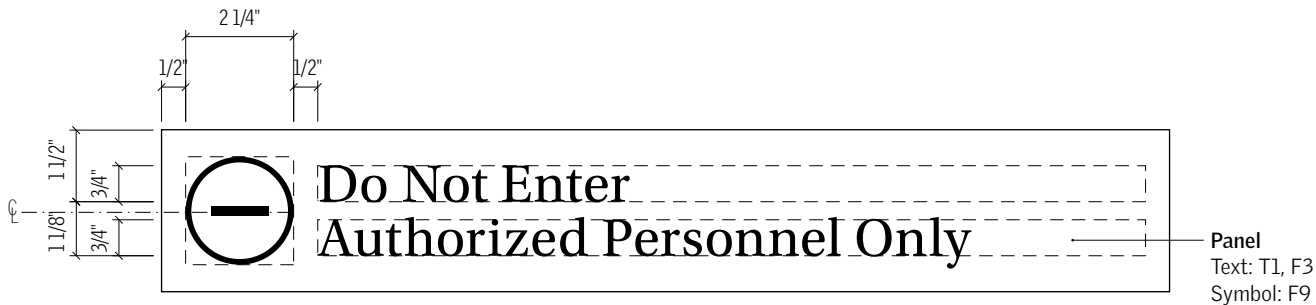
2 Detail Elevation - Sign Type W3 3" = 1'-0"
