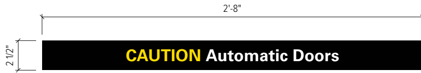
1 Elevation - Sign Type W10 (Door Side 1) 1 1/2" = 1'-0"
