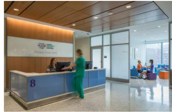
Recycled content included in terrazzo flooring FSC certified wood panel walls and ceiling
